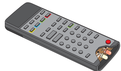
Figure 1.25 The LEDs built into a remote control handset
