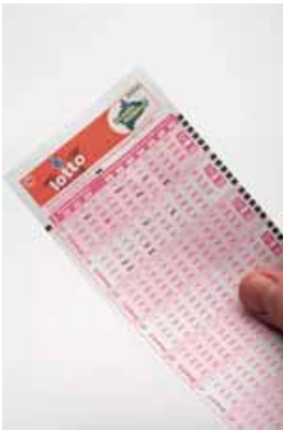
Figure 1.17 A UK National Lottery form. An OMR reader is used to input the information on the form
