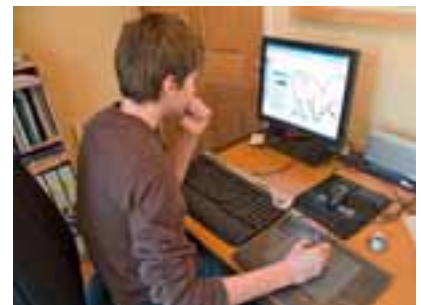
Figure 1.15 Graphics tablet and puck being used to trace a drawing
