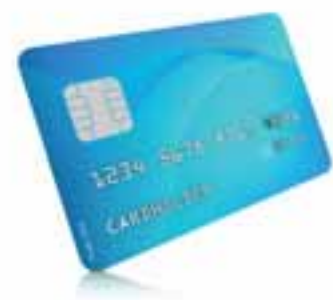
Figure 1.20 A smart card showing the microprocessor chip embedded in it
