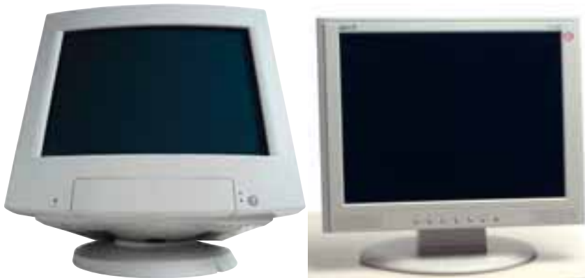
Figure 1.27 Front view of a CRT monitor and an LCD monitor
