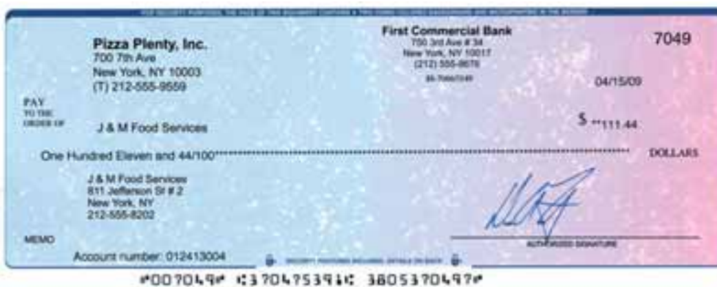
Figure 1.18 MICR uses uniquely shaped characters, printed in magnetic ink
